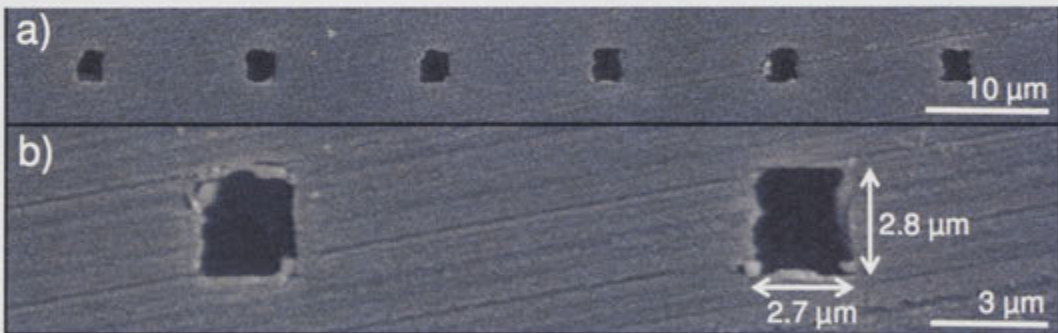
Figure 2.2: SEM micrographs of the cross-section of the diced (a) waveguide array and (b) two waveguides from the array.
